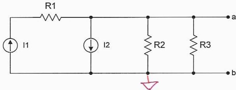
$$V_T = \frac{R_2 R_3}{R_2 + R_3} (I_1 - I_2)$$
