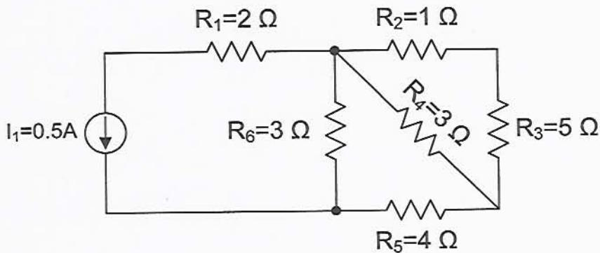
Calculate the numerical value of the power delivered to the circuit by the source  $I_1$ . Write down intermediate results and do not forget the unit.
