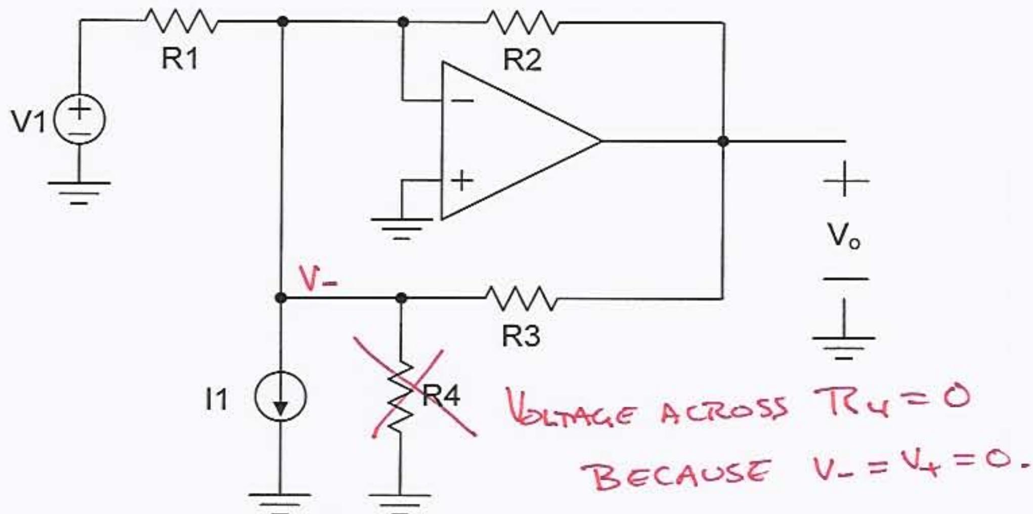
$$V_o = \frac{R_2 R_3}{R_2 + R_3} \left( I_1 - \frac{V_1}{R_1} \right)$$
