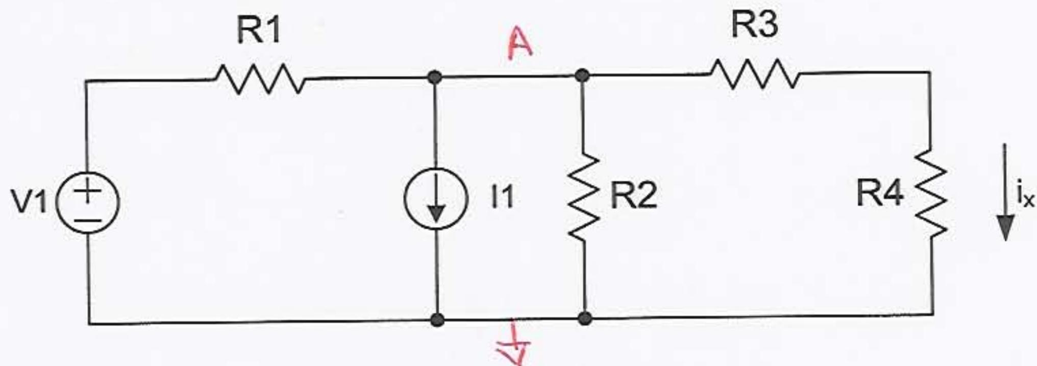
$$i_x = \left( \frac{V_1}{R_1} - I_1 \right) \frac{R_1 R_2}{(R_1 + R_2)(R_3 + R_4) + R_1 R_2}$$
