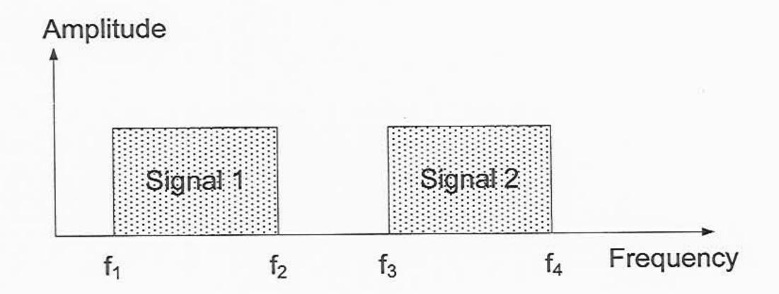
A condition for this to work is that the signals are bandlimited. Signal 1, for example, must not contain energy at frequencies higher than  $f_3$  to avoid corrupting signal 2. This is accomplished by passing signal 1 through a filter H(s). Assuming this filter has a frequency response
