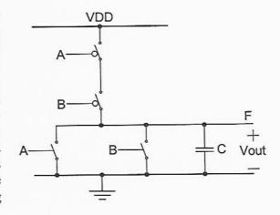
Derive an algebraic expression for the time  $\Delta t$  it takes for  $V_{out}$  to transition from 0V to  $V_{dd}(1-\frac{1}{e})$  (constant  $e \approx 2.718$ ).
