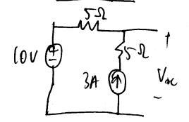
$$3A = \frac{V_{oc} - 10}{5} \Rightarrow V_{oc} = 25V$$
