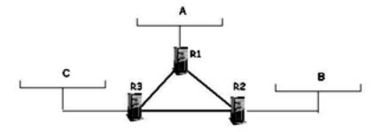
Assign IP addresses to the six subnets in the figure from the block 255.255.255/23. Ethernets A and B should have enough addresses to support 120 interfaces, and C requires enough to support 250 interfaces. Make sure to assign a sufficient number of addresses to the remaining three subnets as well.
