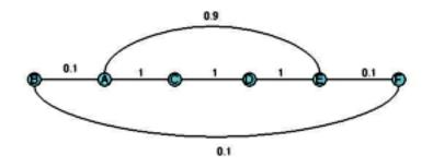
(\*) Assume that time is slotted (t=1,2,3...) and that a node sends its distance vector estimates to its neighbors at the beginning of each slot. A distance vector estimate sent at the beginning of a slot arrives by the end of that slot. All distance estimates are computed using the most recently available estimates.
