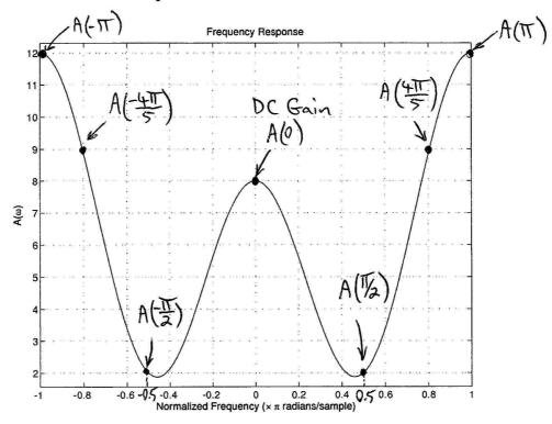
The frequency axis in the figure is normalized by  $\pi$ ; hence, for example, the normalized frequencies 0.5 and 1 refer to  $\omega=\pi/2$  and  $\omega=\pi$  radians per sample, respectively.
