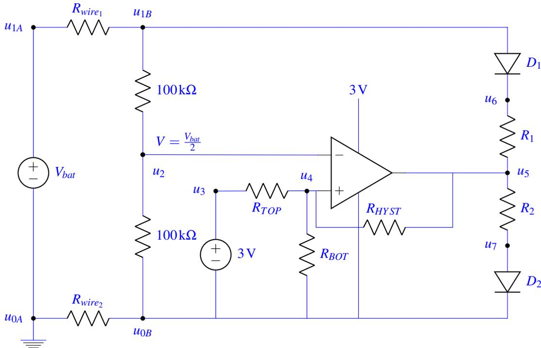
We solve this circuit with superposition, first setting the 3 V source to 0 V, and then setting the output of the comparator to 0 V:
