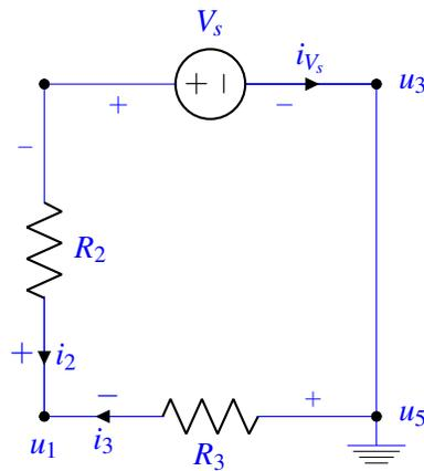
$$i_b = \frac{V_s}{R_3 + R_2} = \frac{4\text{V}}{2\Omega + 3\Omega} = 0.8\text{ A}$$
