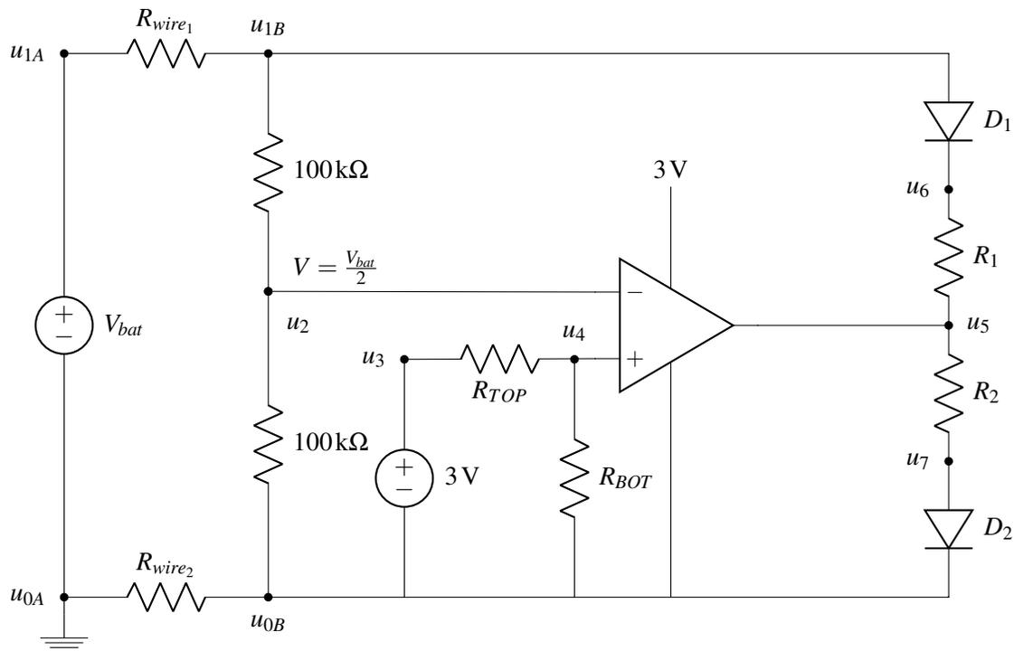
You suspect that there might be a sudden change in the voltage drop across these wires that reduces the voltage (nominally  $\frac{V_{bat}}{2}$ ) at the  $V^-$  input of the comparator when toggling between the two LEDs. Ignoring any hysteresis provided by the comparator, you decide to add your own hysteresis to try to solve the flashing problem.
