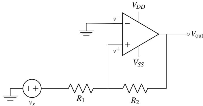
Determine  $v^+$  as a function of  $v_s$  and  $V_{out}$  and other passive components.
