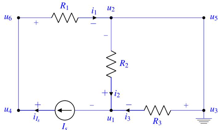
This circuit is a current divider, where  $I_s$  reaches  $u_3$  and then splits such that the voltage across each parallel branch remains constant.
