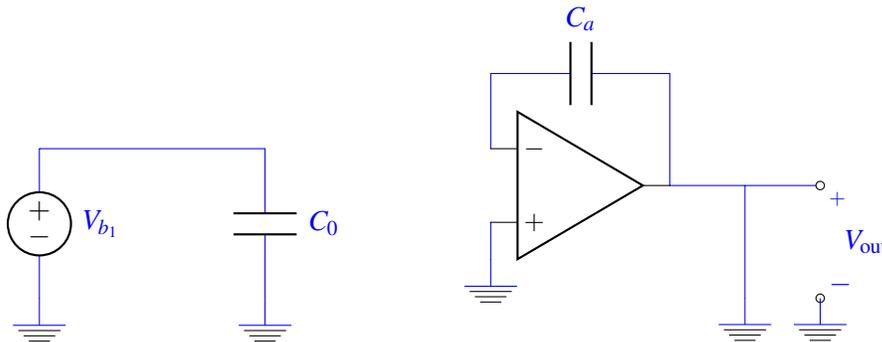
Capacitor  $C_0$  charges from the voltage source:  $Q = V_{b1}C_0$ . With  $\phi_1$  closed,  $V_{out}$  is shorted to ground, and therefore  $V_{out} = 0\ \text{V}$ .
