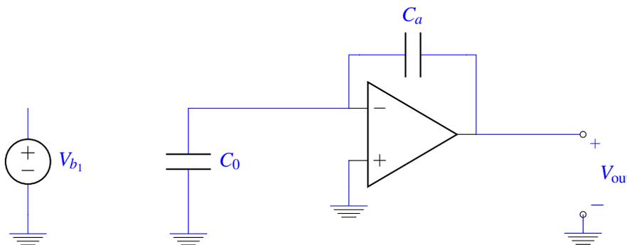
The charge  $Q$  from phase 1 is now shared between  $C_0$  and  $C_a$ :
