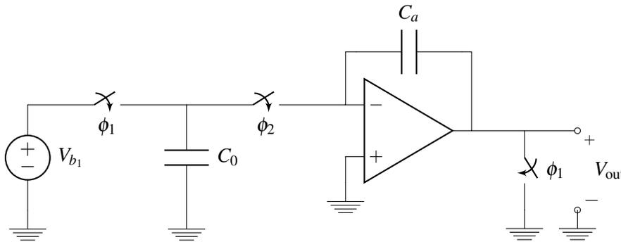
During phase 1,  $\phi_1$  is closed and  $\phi_2$  is open. During phase 2,  $\phi_1$  is open and  $\phi_2$  is closed. What is the voltage  $V_{out}$  during phase 1 and phase 2? You can assume that a long time has passed in each phase before  $V_{out}$  is measured.
