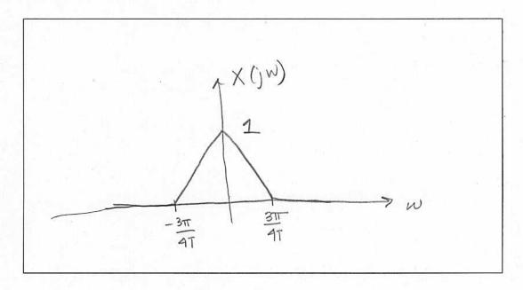
3. (b) 5 points For the same x(t) as in part (a), suppose the A/D converter is now operated at  $\frac{1}{T_1} = 160 \; kHz$  to produce  $x_1[n]$ . Plot the spectrum of  $x_1[n]$ .
