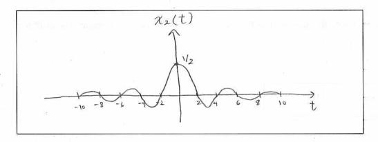
2. (b) 8 points Plot the continuous-time Fourier transform of x(t). Label your axes clearly and carefully!
