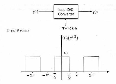
If y[n] is the input to an ideal D/C running at  $\frac{1}{T}=40~kHz$ , and y[n] has the spectrum shown in the figure above, plot  $Y(j\omega)$ , the spectrum of y(t).
