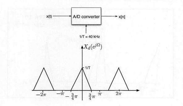
3. (a) 5 points x(t) is sampled above its Nyquist rate at  $\frac{1}{T}=40~kHz$  to produce x[n] whose spectrum,  $X_d(e^{j\Omega})$ , is shown in the figure above. Plot  $X(j\omega)$ , the spectrum of x(t), clearly labeling your axes.
