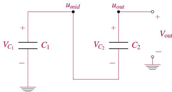
We can see that during phase 2 there are two floating nodes:  $u_{mid}$  and  $u_{out}$ .
