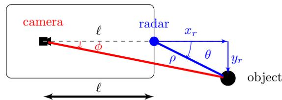
Figure 23: Sensor Placement and Offset  $\ell$ .
