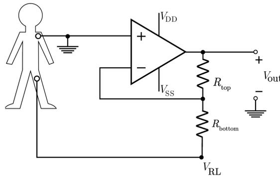
Figure 8: Alternative op-amp ECG topology with  $V_{in}$  zeroed-out
