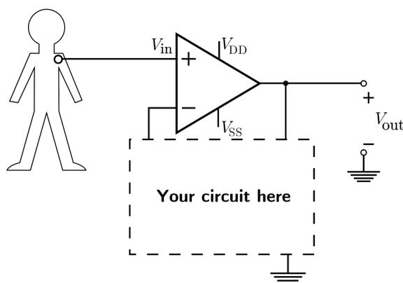
Figure 4: Unfinished ECG amplification circuit.
