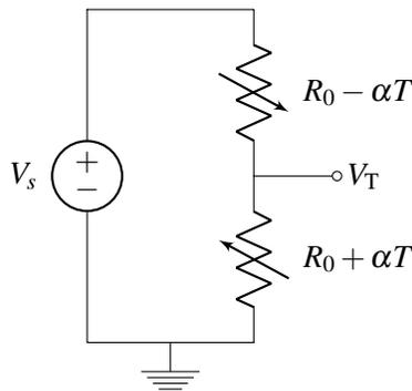
Figure 20: Temperature Sensing Circuit
