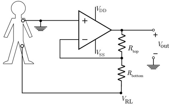
Figure 9: Alternative op-amp ECG topology with  $V_{RL}$  zeroed-out
