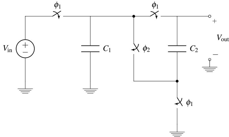
Figure 10: Switch capacitor voltage boosting circuit.
