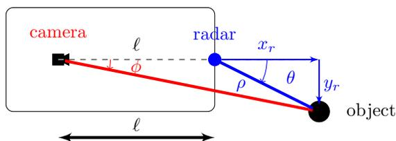
Figure 20: Sensor Placement and Offset  $\ell$ .
