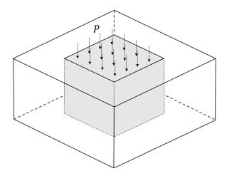
(a) Let  $\epsilon$  be the extensional strain in the inserted material in the direction perpendicular to its exposed face. Find the constant C in the relation
