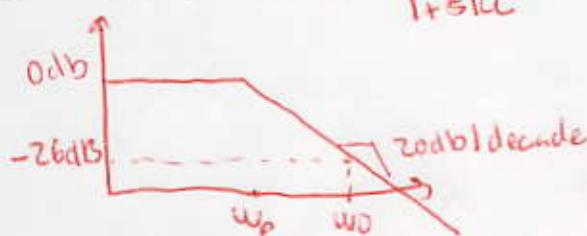
The transfer function of a first-order system is given by  $H(j\omega) = \frac{1}{1 + j\omega RC} = \frac{1}{1 + j\omega w_p}$ . If  $\omega \gg w_p$  (large), the imaginary term in the denominator dominates, and we have
