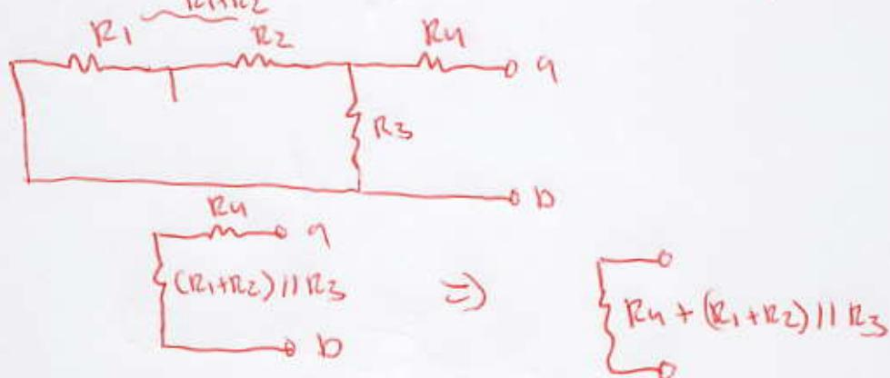
$$R_L + (R_1 + R_2) \parallel R_3 = R_L + \frac{R_3(R_1 + R_2)}{R_1 + R_2 + R_3}$$
