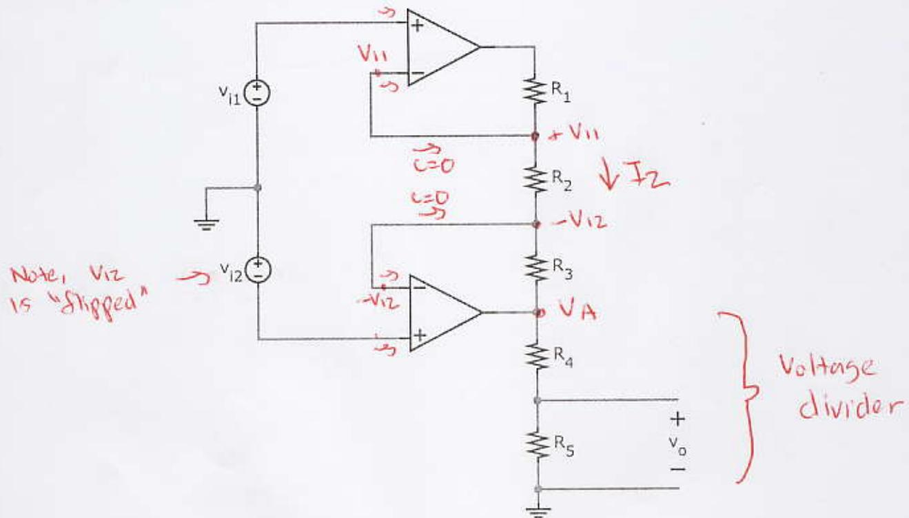
$$v_o = -\frac{R_5}{R_4+R_5} \left[ V_{i2} + (V_{i1} + V_{i2}) \cdot \frac{R_3}{R_2} \right]$$
