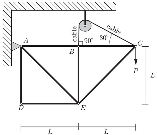
1. Determine the tension in the cable and the forces in all the members of the truss for the loading shown (a vertical force  $P$  at joint C).
