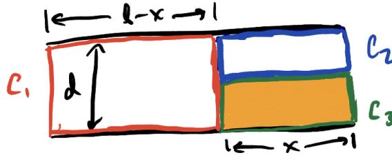
Capacitors  $C_1$  and  $C_2$  are parallel plate capacitors with no dielectric media,  $C_1$  having plate area  $\ell(\ell - x)$  and plate separation  $d$  and  $C_2$  having plate area  $\ell x$  and plate separation  $d/2$ . Capacitor  $C_3$  is a parallel plate capacitor with dielectric media  $K$ , plate area  $\ell x$ , and plate separation  $d/2$ . With these specifications, then
