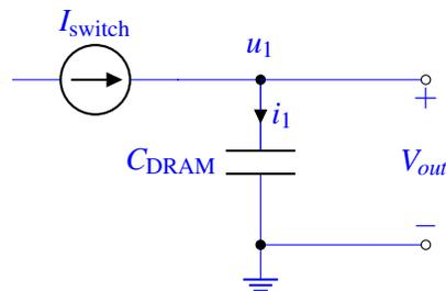
A single KCL equation at node  $u_1$  gives  $I_{\text{switch}} = i_1$ , where  $i_1 = \frac{dQ}{dt} = C_{\text{DRAM}} \frac{dV_{\text{out}}}{dt}$ . We integrate and solve for  $V_{\text{out}}(t)$  at  $t = 1 \text{ ms}$  as follows:
