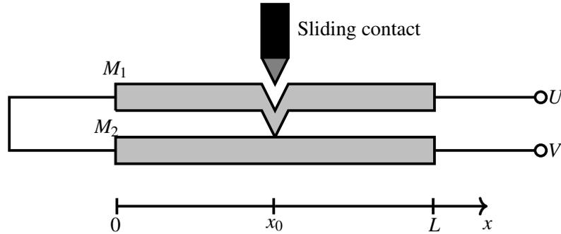
Figure 5.2: Sliding switch making a contact between  $M_1$  and  $M_2$ .
