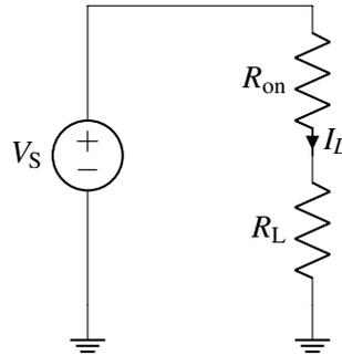
Figure 4.2: Resistive load bank in a circuit with a non-ideal switch.
