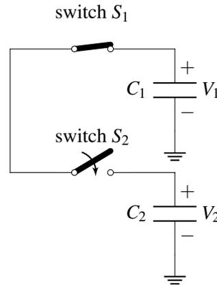
Figure 8.6: Two DRAM cells in parallel. Switch  $S_1$  is closed (can be thought of as a wire), and switch  $S_2$  is closing.
