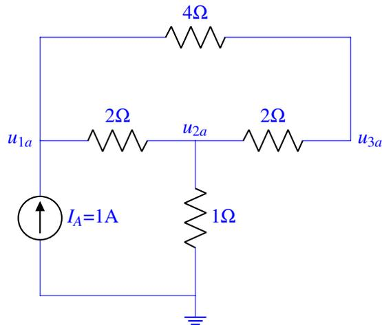
We show one solution approach using series/parallel equivalence and Ohm's law. We can redraw this circuit as follows:
