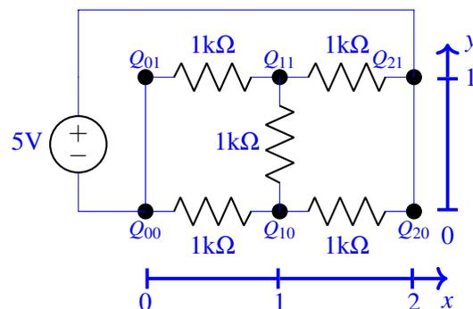
Another acceptable configuration is shown below. Voltages at  $x=2$  (i.e.  $Q_{20}$  and  $Q_{21}$ ) are all 4V and at  $x=0$  (i.e.  $Q_{00}$  and  $Q_{01}$ ) are all 0V. Voltages at  $x=1, y=0$  (i.e.  $Q_{10}$ ) is 3V and at  $x=1, y=1$  (i.e.  $Q_{11}$ ) is 5V. Note that each  $x$ -coordinate has at least one unique voltage, we we can determine the  $x$ -axis.
