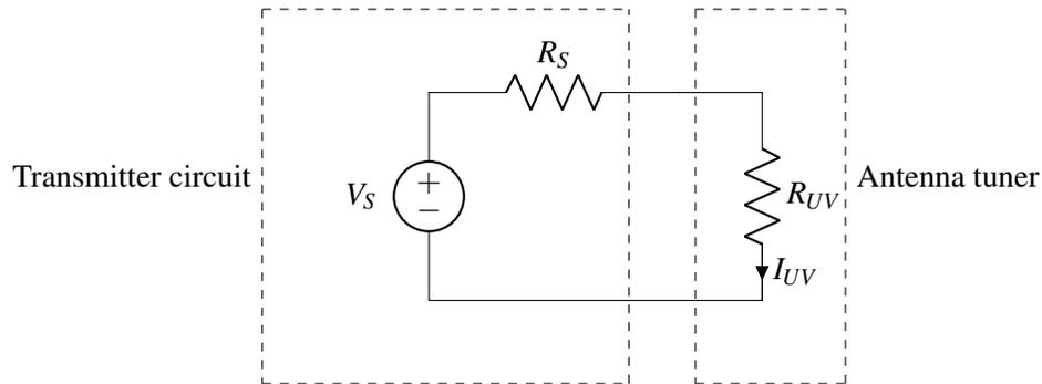
Figure 5.3: Circuit model for the radio transmitter.
