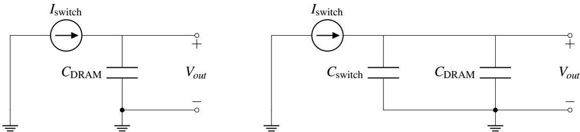
Figure 8.3: Left: Circuit without parasitic capacitance. Right: Circuit with parasitic capacitance.
