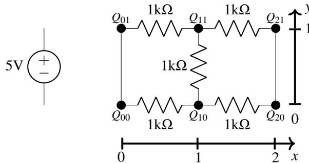
Figure 6.3: Resistor grid for part (d).
