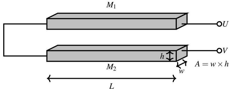
Figure 5.1: Resistive metal bars connected through ideal wires.
