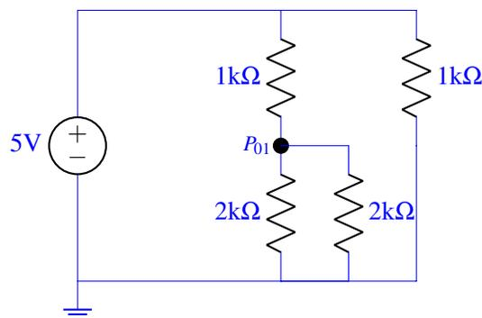
Note that we have two parallel resistors, each of  $2k\Omega$ , connecting  $P_{01}$  to ground. We can therefore re-draw the circuit as:
