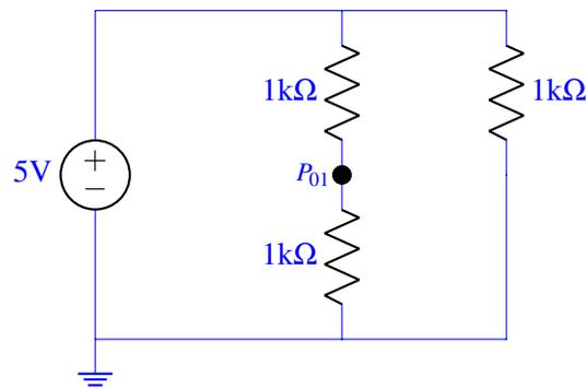
We can therefore solve for the voltage at  $P_{01}$  as a voltage division of 5V:  $P_{01} = 5V \frac{1k\Omega}{1k\Omega+1k\Omega} = 2.5V$ . No other point on the circuit has this voltage. Therefore, yes, we can identify where the touch happened, and we can do so uniquely as there is only one point that exists with this voltage:  $P_{01}$ .
