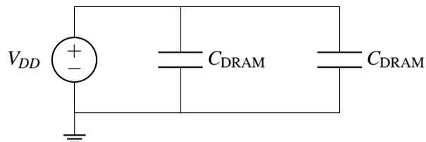
Figure 8.4: DRAM capacitors in parallel are charged.
