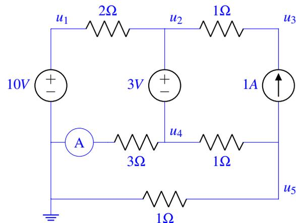
Figure 3.6: Ammeter placement to measure current flowing through the  $3\Omega$  resistor.
