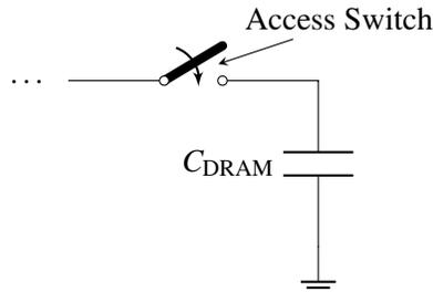
Figure 8.1: A DRAM cell consisting of an access switch and a capacitive storage element,  $C_{DRAM}$ .
