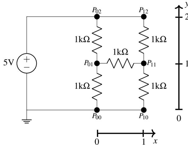
Figure 6.1: A schematic of the H-shaped resistive touchscreen.
