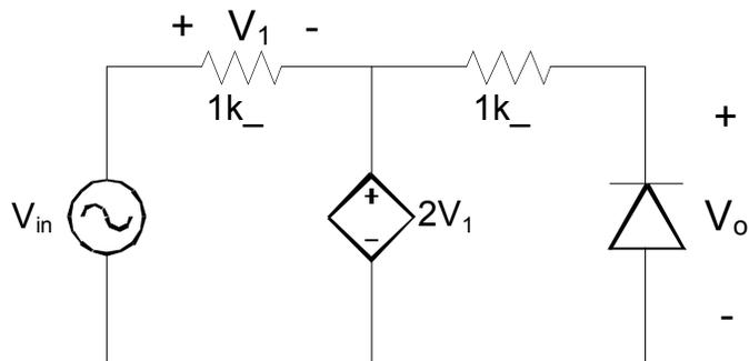
(i) (4 pts) Re-draw the circuit assuming the diode is off. Express  $V_o$  as a function of  $V_{in}$ .
