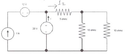
(c) Find the Norton equivalent of the circuit below at the AB terminal. (Hint: Use source transforms to quickly solve this problem) (10 points).
