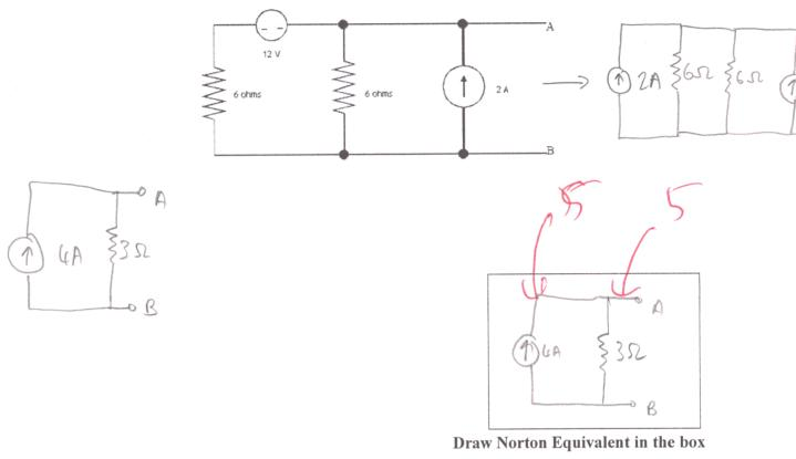
(d) Find the Thevenin equivalent of the circuit below at the AB terminal (10 points).
