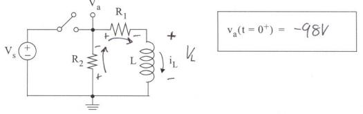
[8 pts.] (e) Determine  $v_a(t)$  for t > 0.  $V_a(t) = V_af + \left[ V_a(o^+) - V_af \right] e^{-t/2}$   $v_a(t) = -98e^{-t \cdot 10^4 \text{ sec}^{-1}}$   $lim V_a(t) = 0$   $t \to \infty$  $V_a(t) = V_a(t) + V_a(t)$
