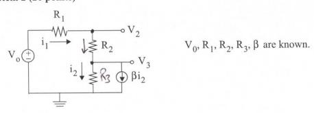
[10 pts.] (a) Write (but do not solve) a minimum set of equations that could be solved for unknowns V<sub>2</sub> and V<sub>3</sub> using Kirchhoff's Current Law, KCL. (Equations in box for full credit.)
