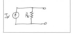
[2 pts.] (d) In general, if you know  $V_{TH}$  and  $R_{TH}$ , how do you determine  $R_N$  and  $I_N$ ?
