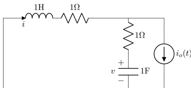
Consider the circuit above with the inductor current  $i$  and capacitor voltage  $v$  as state variables and with the independent current source  $i_o$  as input.
