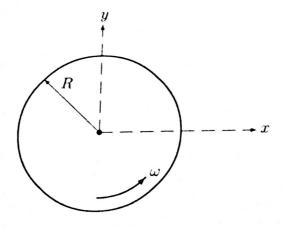
A thin disk of radius R is lying on the xy-plane, centered at the origin. It carries a uniform surface charge density  $\sigma$  (with total charge  $Q = \pi R^2 \sigma$ ) and is spinning with angular velocity  $\omega$  (around the z-axis). Find an expression for that magnetic field  $\vec{B}$  far away from the disk (at distance  $r \gg R$ ).
