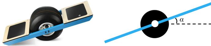
One challenge of building a one-wheel scooter is designing a circuit that measures the angle  $\alpha$  of the riding platform, as shown above. You are considering the design of an angle sensor consisting of two capacitors  $C_a$  and  $C_b$  whose values depend on the angle  $\alpha$  (measured in degrees) as follows:
