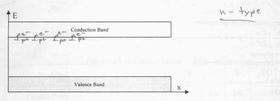
**c)** (6 pts.) The Si from part b) is doped with an additional  $6x10^{17}$  B atoms-cm<sup>-3</sup> (so the Si is doped with P and B). Now what type is the Si? Redraw the energy level diagram, showing how both impurities ionize.
