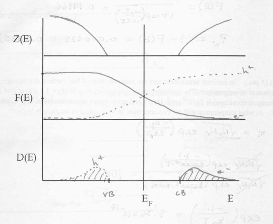
b) (3 pts.) For intrinsic semiconductors the Boltzmann tail approximation is typically used in which  $F(E) \approx \exp(-\frac{E - E_F}{kT})$ . Show how this approximation is valid.
