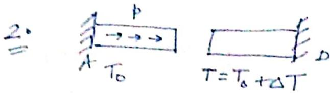
a)  $\frac{T < T_1}{\sigma_A = \frac{p \cdot L}{A}} \quad \sigma_B = 0 \text{ (no constraint yet)}$
