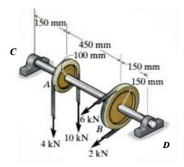
b) The same arrangement is again set up for a shaft made of a single material with an unknown but constant G. Give a brief explanation of how you would determine G experimentally.
