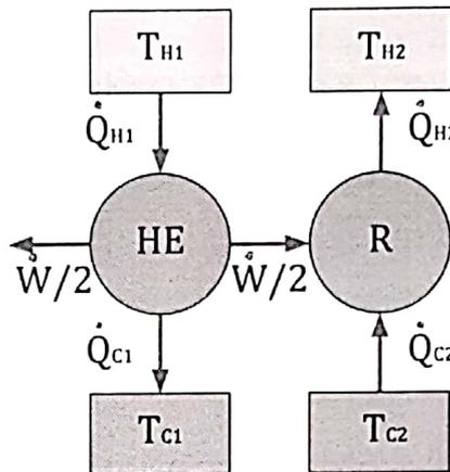
One-half of the power output of this heat engine is used to drive a refrigerator that removes heat from the cold freezer cabinet at  $T_{C2} = -5 \text{ }^\circ\text{C}$  and transfers it to a kitchen at  $T_{H2} = 22 \text{ }^\circ\text{C}$ . The inventor tells you that the heat engine / refrigerator system design is capable of removing heat at a rate of  $\dot{Q}_{C2} = 6.25 \text{ kW}$ .
