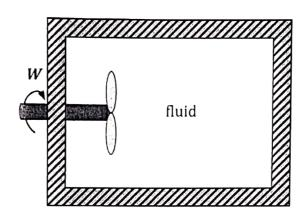
If the fluid temperature and pressure are initially 20 °C and 100 kPa respectively, what is the change in specific internal energy,  $\Delta u$ , caused by the work interaction from the propeller rotation if the fluid is:
