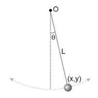
c) (5) Derive the transfer function  $\frac{\theta(s)}{\theta_0}$  for the pendulum above, where  $\theta_0$  is a non-zero initial angle of the pendulum.
