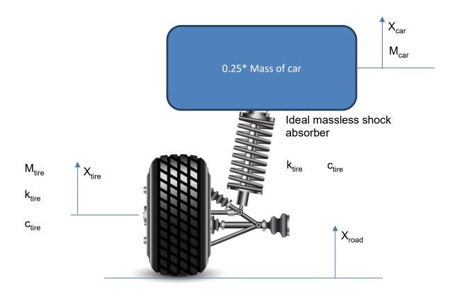
b) (5) Assuming the mass of the car is infinite, reduce the model to a  $2^{nd}$  order system. Derive the State Space model for the new  $2^{nd}$  order system
