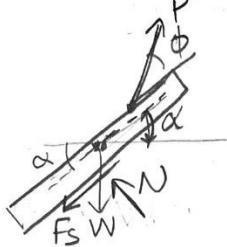
Along the inclined plane right before the pipe starts moving we have  $\sum F = 0$  and  $F_s = \mu_s N$ , therefore
