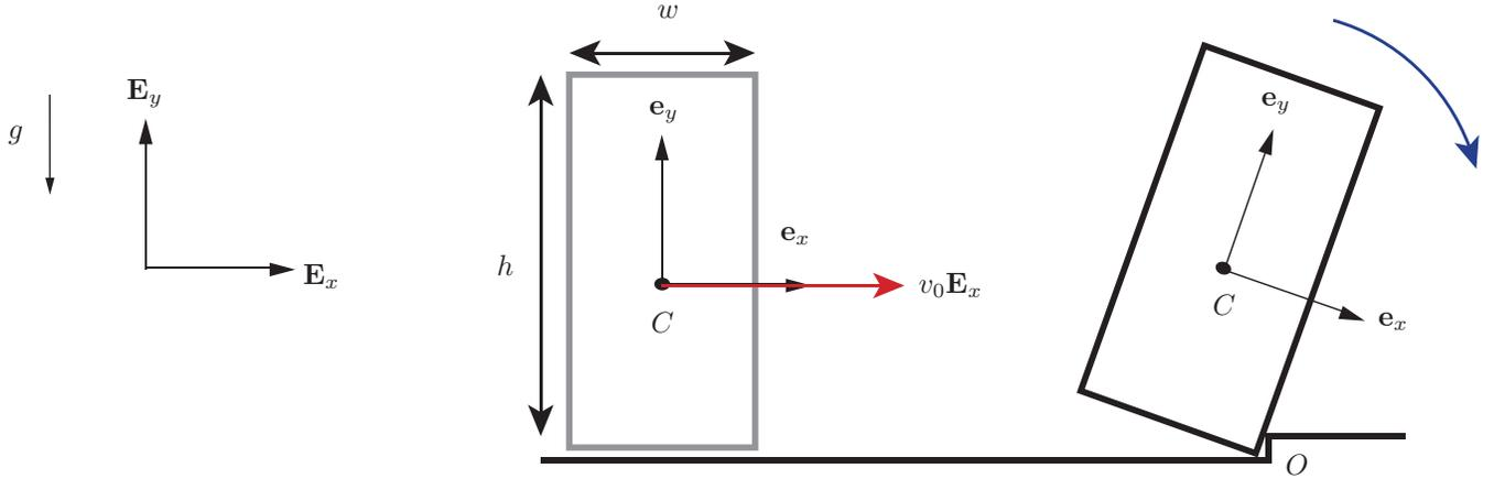
Figure 3: A rigid body of mass  $m$  moves atop a smooth horizontal surface and collides with a ledge at  $O$ . After the impact the rigid body rotates about  $O$ .
