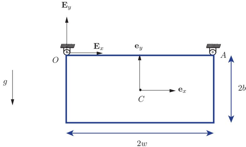
Figure 1: A rigid body of mass  $m$  is free to rotate about  $O$  (after the pin joint at  $A$  is released) and is subject to a gravitational force.
