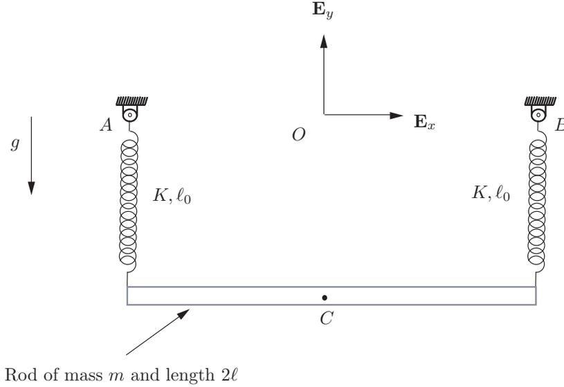
Figure 4: A uniform rod of length  $2\ell$  is suspended by two identical linear springs. The rod is free to move on a smooth vertical plane.
