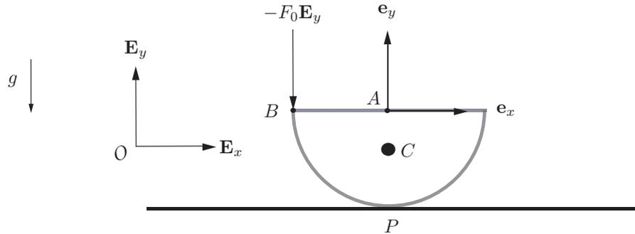
Figure 2: A rigid semicylinder of mass  $m$  and radius  $R$  moving on a horizontal plane. A constant force  $-F_0\mathbf{E}_y$  acts at a point  $B$  on the semicylinder.
