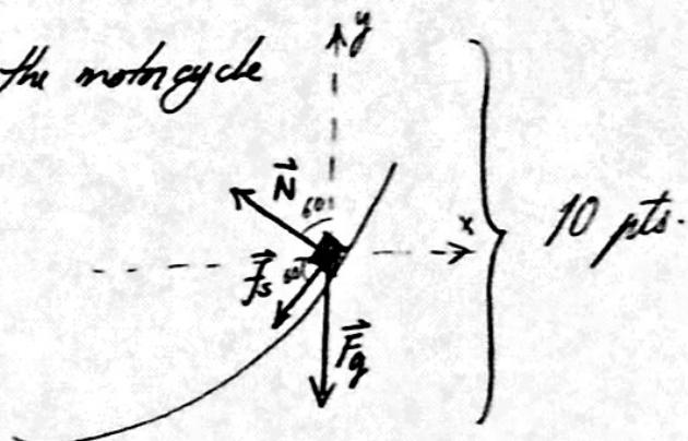
When the motorcycle is about to slide out, friction points inward
