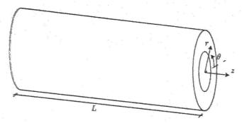
In this setting the temperature is only a function of radial position, r, and polar angle  $\theta$  and the temperature  $T(r,\theta)$  can be determined by solving a two-dimensional problem in the  $r,\theta$ -plane that is governed by the weak form equation
