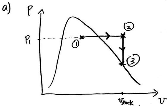
b). Initially, constant pressure heat addition, when  $V = V_{\text{lock}}$ , constant volume heat removal.
