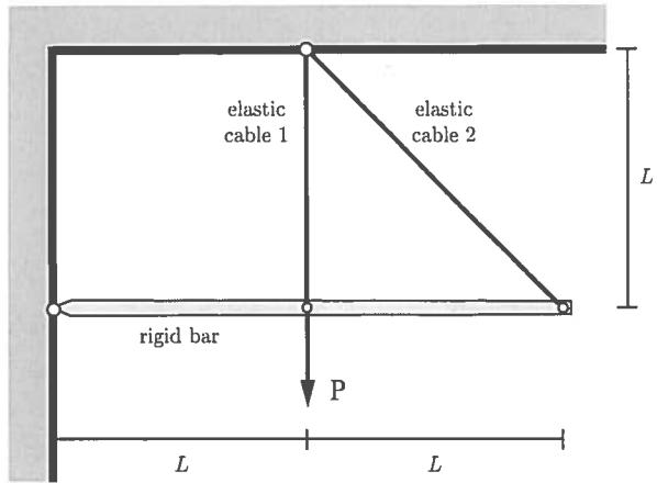
Statically indeterminate  $\Rightarrow$  Force method
