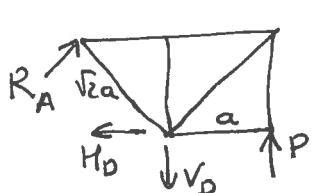
$$\begin{aligned} (\sum M_D = 0) &\Rightarrow R_A \sqrt{2}a = Pa \Rightarrow R_A = \frac{P}{\sqrt{2}} \\ (\sum F_{\text{hor}} = 0) &\Rightarrow H_D = R_A \cos 45^\circ = \frac{P}{2} \\ (\sum F_{\text{vert}} = 0) &\Rightarrow V_D = R_A \sin 45^\circ + P \Rightarrow V_D = \frac{3P}{2} \end{aligned}$$
