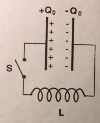
An L-C circuit consists of a coil of an inductor with self-inductance L and a capacitor, of capacitance C. The capacitor plates initially have charges  $\pm$  Q<sub>0</sub>. The switch S is initially open and is then closed at time t = 0. Express your answers in terms of Q<sub>0</sub>, L, C, and t.
