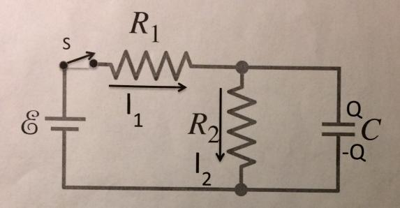
In the RC circuit above, after the switch is closed at time t=0, currents  $I_1$  and  $I_2$  flow through the resistors  $R_1$ ,  $R_2$ , and the capacitor C has a charge Q(t). The capacitor C is initially uncharged: Q(t=0)=0.
