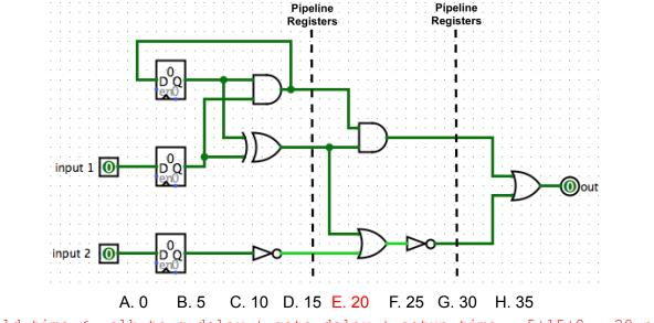
Hold time  $\leq$  clk-to-q delay + gate delay + setup time = 5+15+0 = 20 ns
