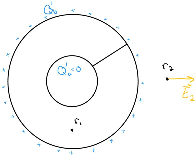
Figure 2: Now that a wire connects the spheres, all excess charge moves to the outer sphere.  $\vec{E}_1$  is now zero, and  $\vec{E}_2$  remains unchanged.
