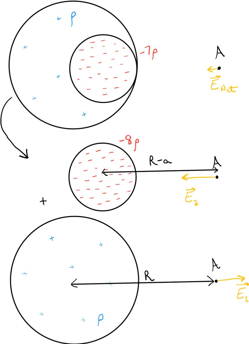
Figure 3: Separation of the original charge configuration into two uniformly charged spheres.
