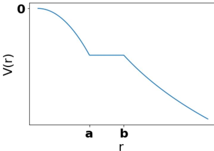
Figure 5: Voltage as a function of  $r$ , the distance from the center. The chosen zero point is marked as  $V(0) = 0$ , but this doesn't really have any physical significance. It's differences in electric potential that physically matter, so the shape of this graph is the important part.
