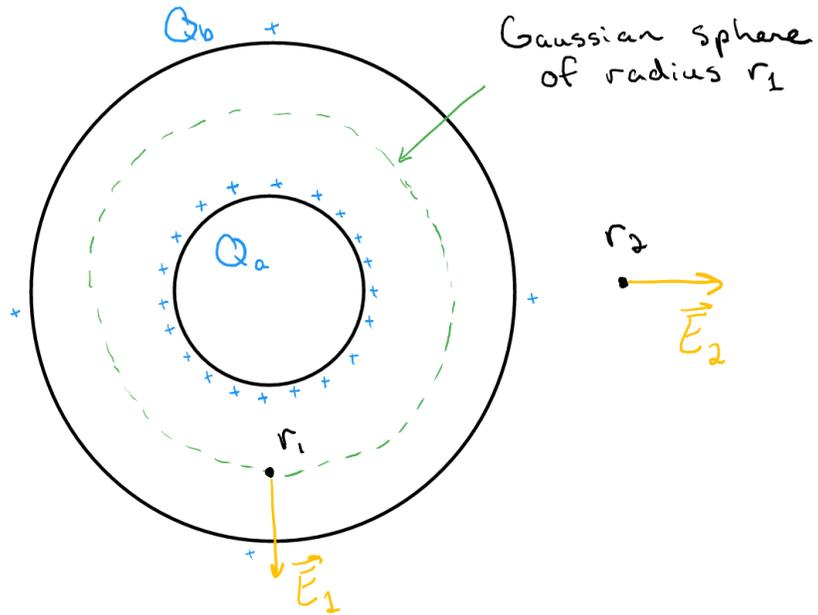
Figure 1: The electric fields for Part A, with the Gaussian surface used to find  $\vec{E}_1$ .
