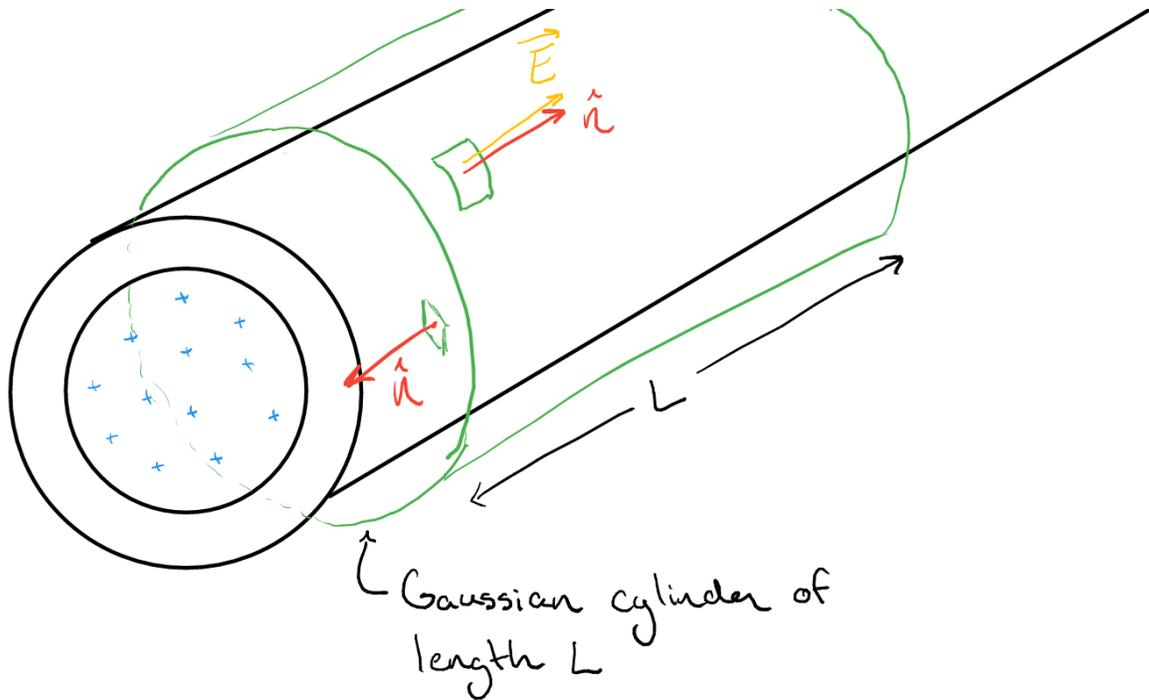
Figure 4: Electric fields pointing radially outward will only ‘pierce’ through the curved side of the Gaussian cylinder. (Surface charge distributions have not been marked on the conducting shell.)
