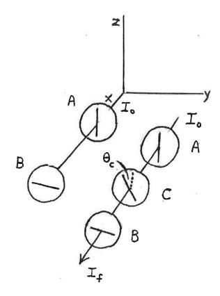
Unpolarized light of intensity  $I_o$  propagates along the x-axis and passes through two polaroid filters, as shown above. The transmission axis of filter A is in the z-direction, while that of B is in the y-direction. The final intensity of light passing through B, which we denote as  $I_f$ , is zero.
