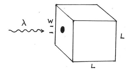
A hollow cube, made of stiff cardboard, has sides of length L. On the face of the cube is a small, circular hole of width W. Monochromatic light of wavelength  $\lambda$  enters the hole and creates a bright, circular spot of diameter S on the opposite face, inside the cube.
