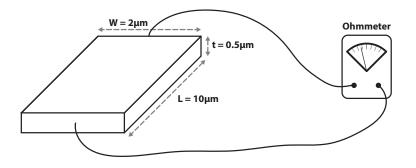
(a) Based on the dimensions shown, what is the resistivity of the sample? The conductivity?
