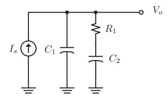
(a) Find the transfer function  $V_o/I_s$  and put into a standard form.
