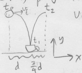
velocity at  $t_0$  &  $t_2$  is purely horizontal. During bounce, the ball experiences a torque about c.m., so its  $\omega$  changes, but the vertical component of  $\vec{v}_{cm}$  has same magnitude before & after.
