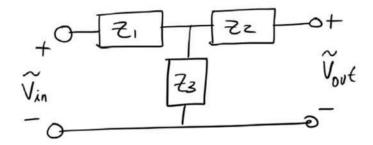
a) Provide an expression for  $\ \widetilde{H}_{out}(\omega)=rac{\widetilde{v}_{out}(\omega)}{\widetilde{v}_{in}(\omega)}$
