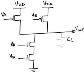
a) Fill in the truth table below for the circuit above.  $V_A$ ,  $V_B$  and  $V_{out}$  are digital voltages that can only assume values of 0 or  $V_{DD}$ . (5 points)
