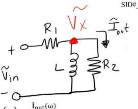
We define a transfer function  $\widetilde{H}_{out}(\omega) = \frac{\tilde{I}_{out}(\omega)}{\widetilde{v}_{in}(\omega)}$ .
