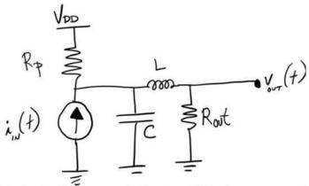
We are going to solve this circuit, which contains both a sinusoidal and a DC source using superposition and phasors.
