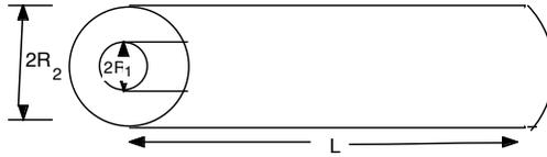
Figure 5: sketch of coaxial cable with dimensions labeled for problem 5. Treat as two concentric cylinders.
