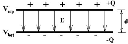
Figure 4: Capacitor shown with ideal field. Draw in necessary fringe field and explain.
