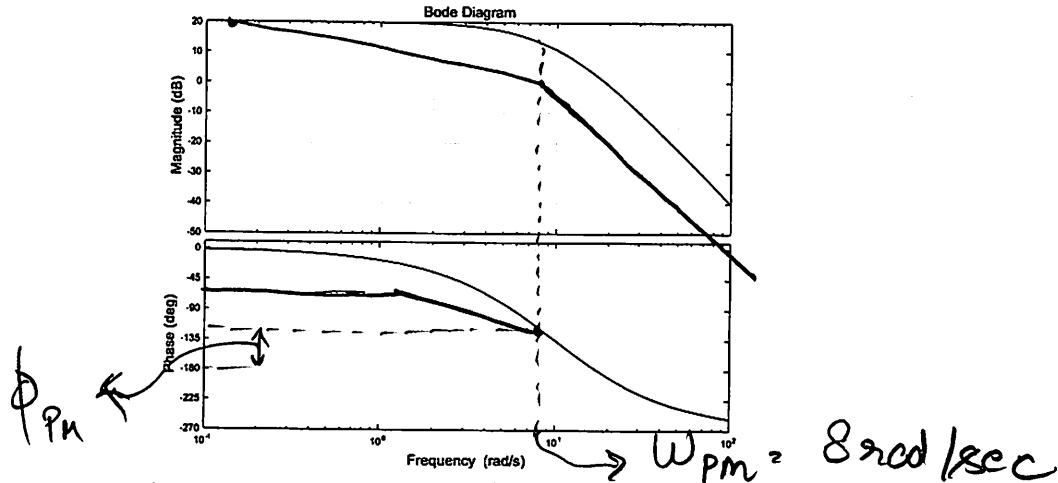
A lag controller  $D(s) = k \frac{s+\alpha}{s+\beta}$  is to be designed such that the unity gain feedback system with openloop transfer function  $D(s)G(s)$  has the same steady state error as with OLTF  $G(s)$  and has a nominal (asymptotic approximation) phase margin  $\phi_m = 55^\circ$  at  $\omega = 8 \text{ rad s}^{-1}$ . Note  $20 \log |G(j\omega = j8)| = 13 \text{ dB}$ .
