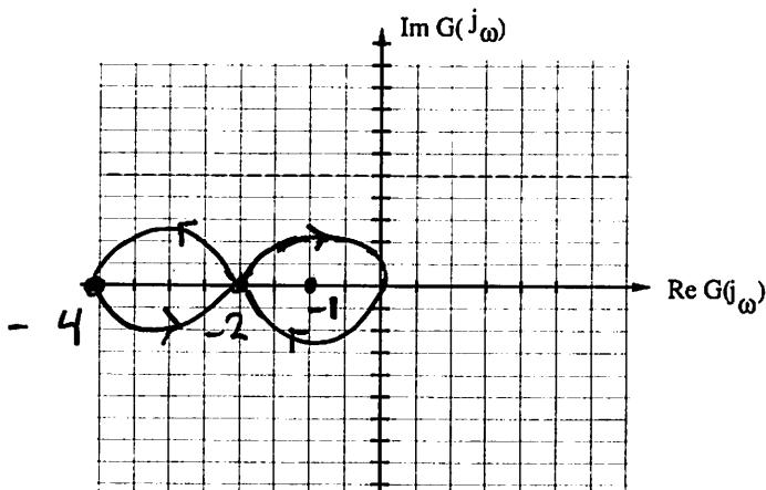
$$\begin{array}{lll} \omega & |G| & \angle G \\ 0 & \frac{16}{4} & \frac{180}{180+180-180} = 180^\circ \\ 1 & \frac{\sqrt{17}}{\sqrt{2}} \approx 3 & \\ 2 & \frac{\sqrt{50}}{\sqrt{5}} = 2 & 180^\circ \\ 6 & \sqrt{\frac{52}{37}} \approx \sqrt{14} \approx 1.2, & \angle \approx -45^\circ + 135^\circ \\ & & -110^\circ + 120^\circ \\ \infty & 0 & \sim 100^\circ \end{array}$$
