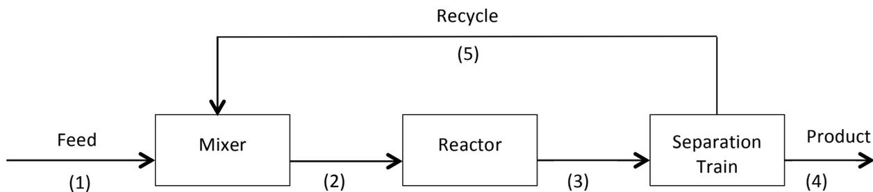
Figure 1. Steady production of aqueous urea from ammonia and carbon dioxide
