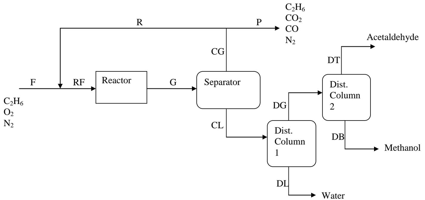
Figure 1. Process flow diagram for production of acetaldehyde from ethane oxidation
