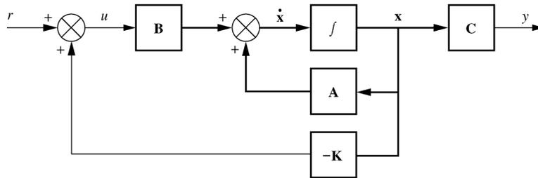
[4 pts] g. Assume the overall control system is stable, and refer to the expanded block diagram above. Describe in words why  $\lim_{t \rightarrow \infty} e_w(t) = 0$  for a step input  $w(t)$ .
