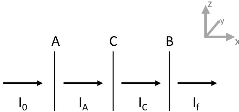
Figure 1: View of polaroid placement, looking in  $+\hat{y}$ -direction, part (a).
