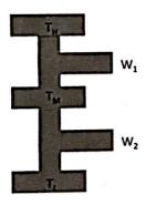
One ideal heat engine with equivalent work output
