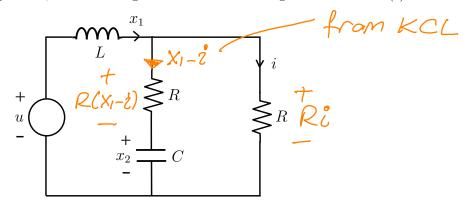
a) (5 points) Write an expression for the current i indicated on the circuit diagram in terms of  $x_1$  (the inductor current) and  $x_2$  (the capacitor voltage). Your answer should **not** involve any derivatives.
