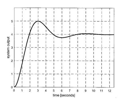
The figure above shows the step response of a second order system with no zeros.
