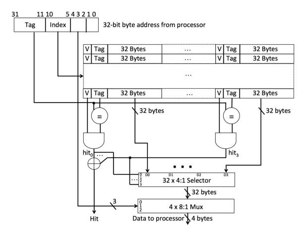
Note: a 4:1 Selector has four control inputs labeled 0, 1, 2, 3 and four data inputs D0, D1, D2, D3. It connects D<sub>i</sub> to the output when the ith control signal is true. Assume that **at most one** control input is true at any time. The selector function is undefined when none of the control inputs are true.
